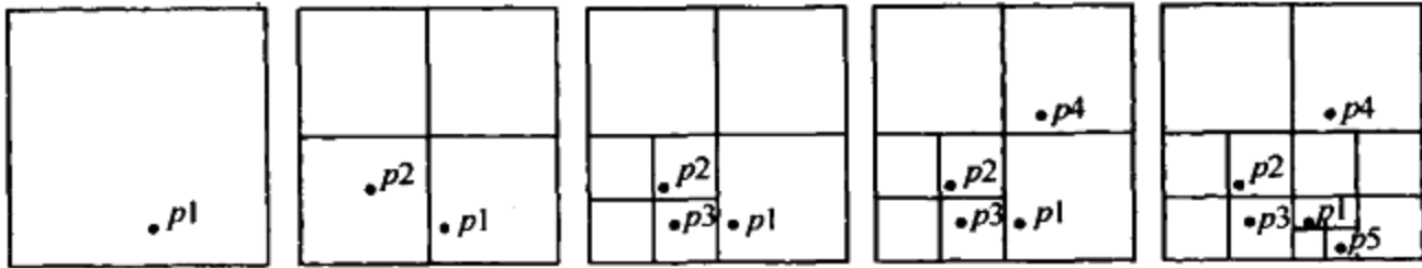
图 12-54 平面由四分树(quad tree)在插入 p_1 = (53, 14) , p_2 = (27, 28) , p_3 = (30, 11) , p_4 = (67, 51) , p_5 = (70, 3) 后所得到的划分
