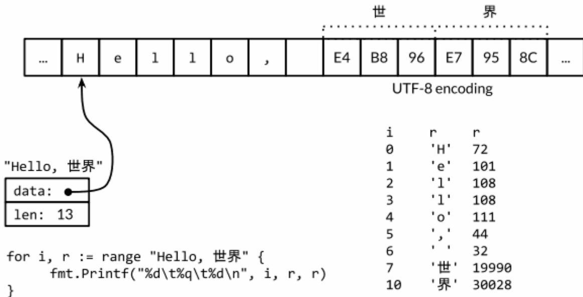
Figure 3.5. A range loop decodes a UTF-8-encoded string.
