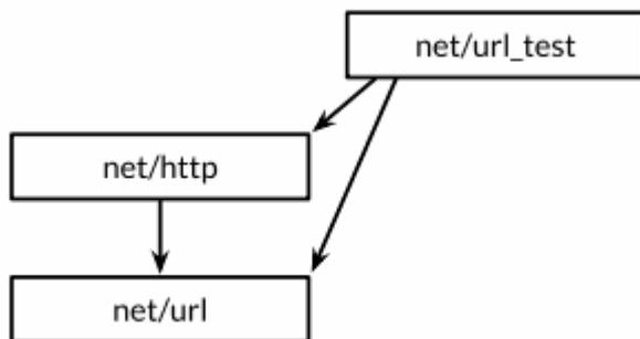
Figure 11.2. External test packages break dependency cycles.
