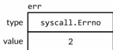
**Figure 7.6.** An interface value holding a `syscall.Errno` integer.
