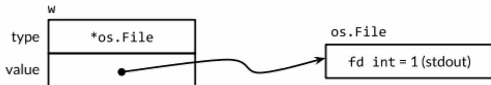
Figure 7.2. An interface value containing an \*os.File pointer.
