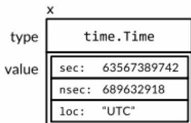
**Figure 7.4.** An interface value holding a `time.Time` struct.
